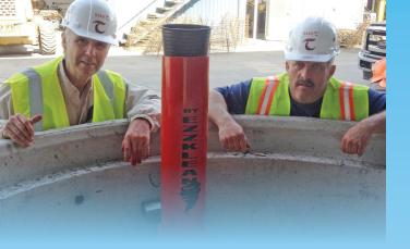
**EZZ-KLEAN™** works to save time during routine maintenance as the wide mouth funnel is always beneath the waste build up and pulling in the debris is made easy i.e. not from the top down as the conventional method would require this method also increases the exposure to injuries as the heavy hose is difficult and cumbersome to handle and the dangers of working over an open hatch exposes the worker to deadly falls.
